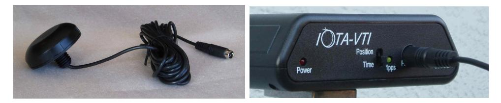
To avoid the exorbitant cost of a custom panel for this low-volume model, a hole is cut in the standard panel. Labels suffer.
